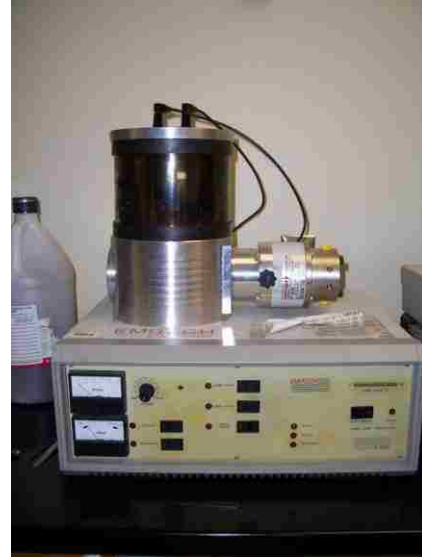
(b) Emtech K950 sputtering machine
