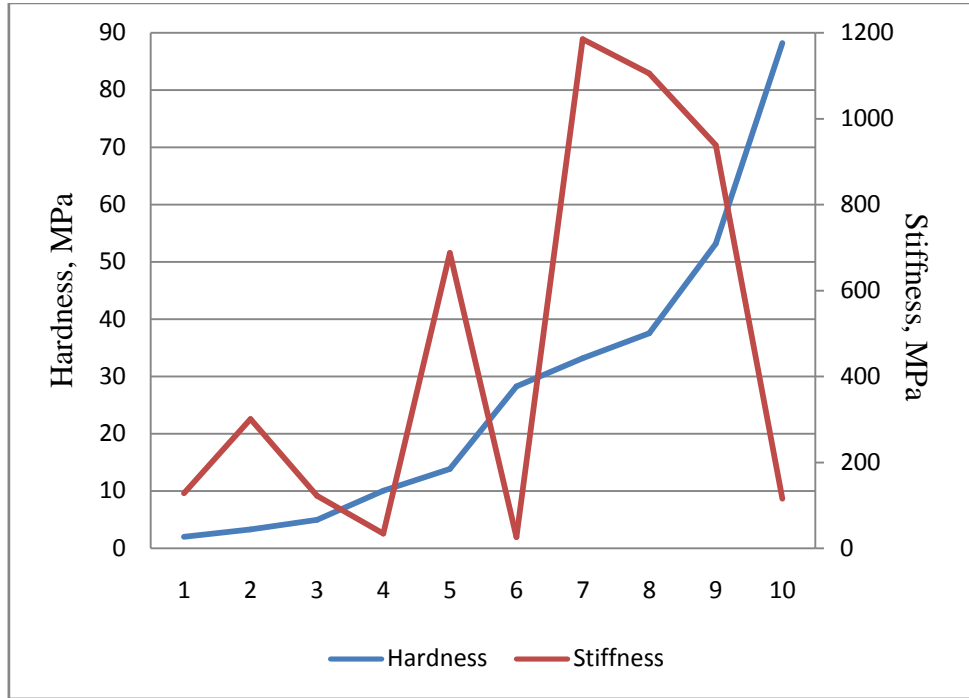
Figure 6.6: Stiffness and Hardness compared to each other, 10% mica mastic, RTFO
