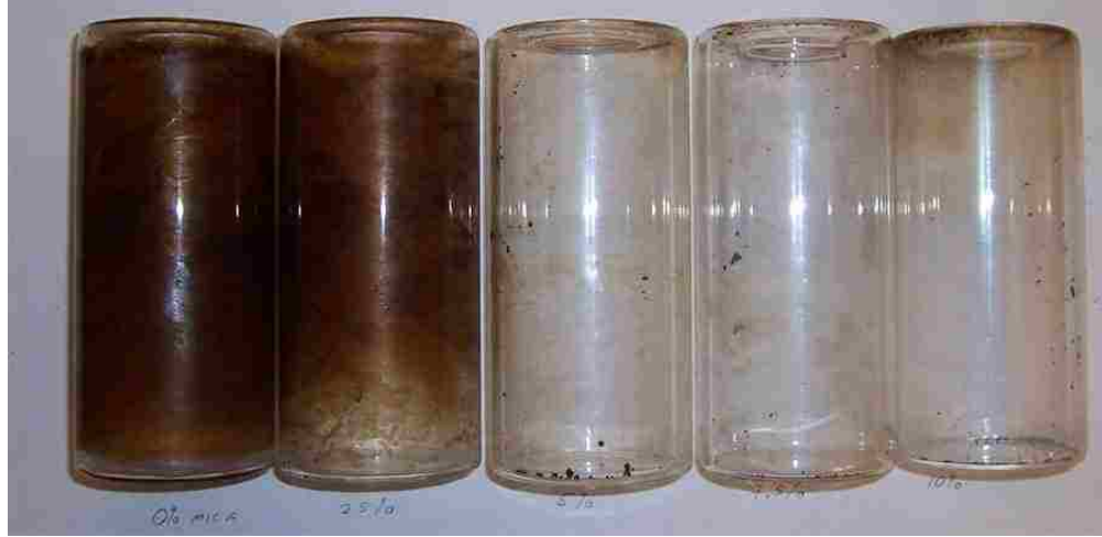
Figure 3.5: RTFO jars from unmodified binder mastic mixes, arranged from 0% to 10% mica
