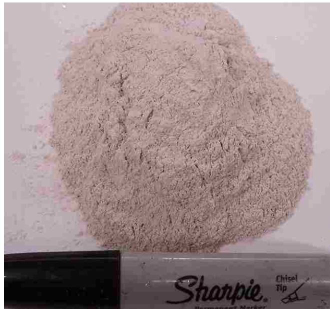
(b) After cleaning, grinding and passing #200 sieve
