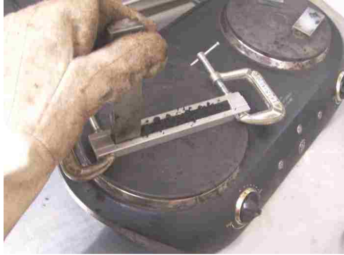
Figure 3.17: Compaction of mastic into mold
