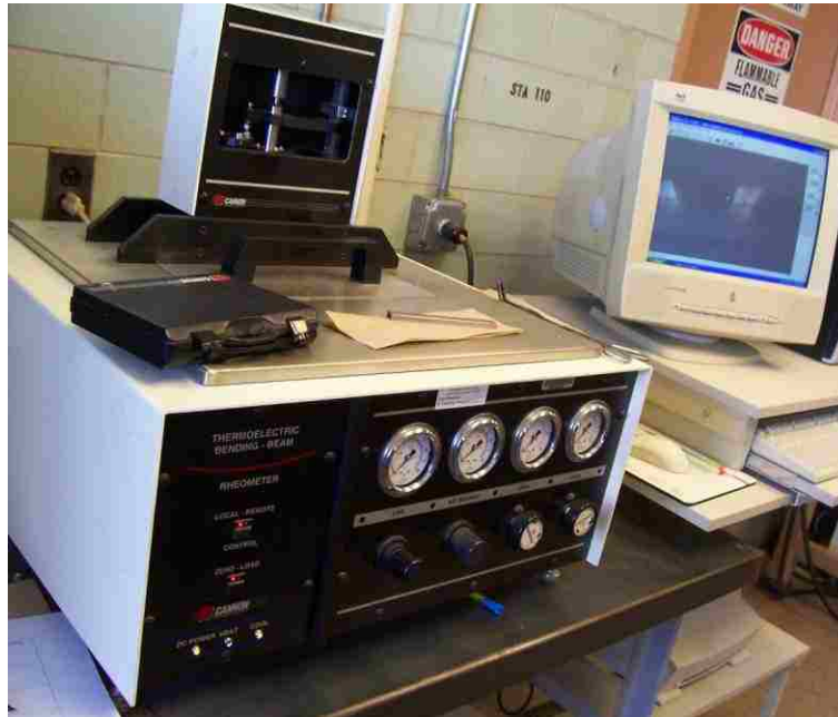
(a) BBR as configured at the New Mexico DOT asphalt test laboratory in Santa Fe, NM
